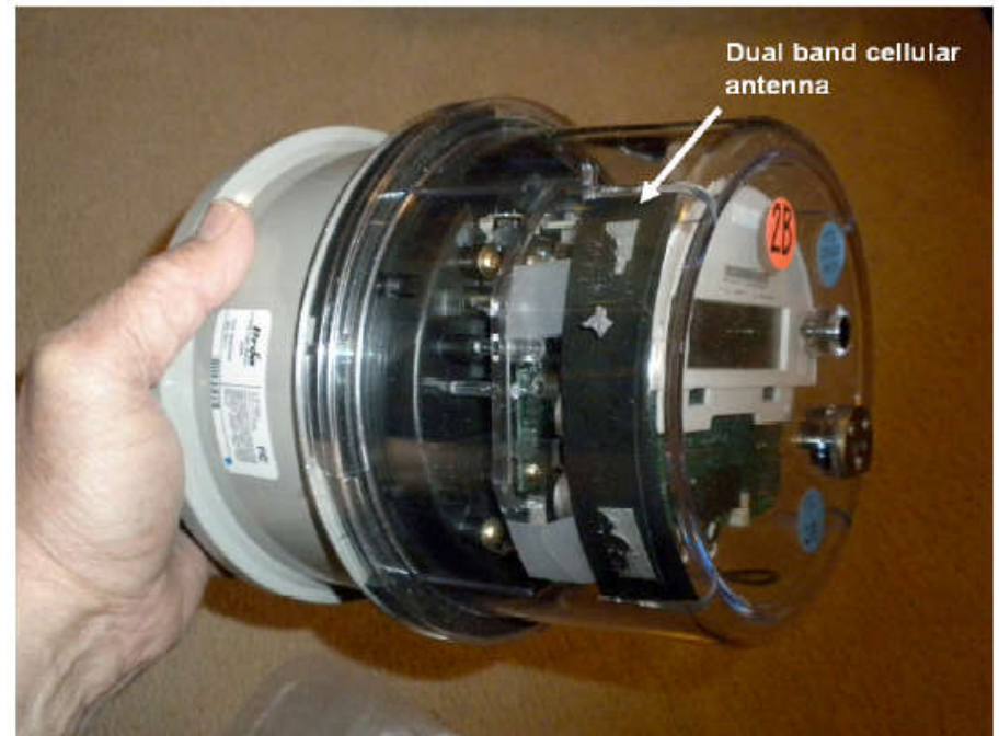
Figure 2-3 Cell relay meter with flexible, dual band (850 MHz and 1900 MHz) antenna affixed to interior surface of the meter cover.
